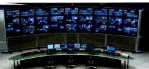
Using multiviewers, the MCR now more resembles a NOC, displaying the screens of playout servers, network traffic and more.
